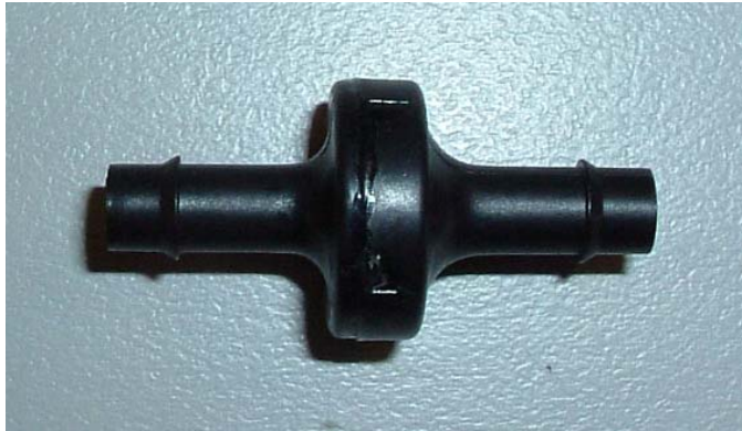
Flap type - 6 mm swage fitting (non spring loaded) Suitable for applications where outputs do not exceed 300mg of ozone per hour.
