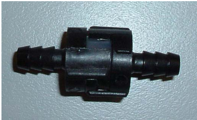
Spring loaded o-ring type – 6mm swage fittings Suitable for applications where outputs do not exceed 4000mg of ozone per hour.
